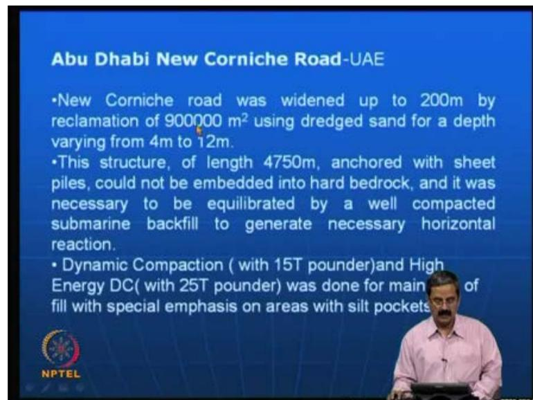
You know it has to, it has, a lot of filling is involved. So, they removed, they got the sand from some places and then they filled up to 4 to 12 meters and the length of the structure is about 4.75 kilometers and actually, it was, it should have been anchored with sheet pile walls. But, it could not be embedded into hard rock and it was necessary to be equilibrated by well compacted submarine backfill to generate necessary horizontal reaction.
