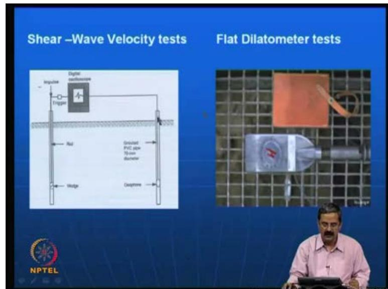
This is a dilatometer; I just mentioned a similar one which in where you have a diaphragm here and then it is a simple kit. Actually, it is a very simple equipment this also has a very versatile application and shear wave velocity measurements. Here again like as I just mentioned whether the dilatometer is also very useful pressuremeter is also very useful and shear wave velocity measurements.
