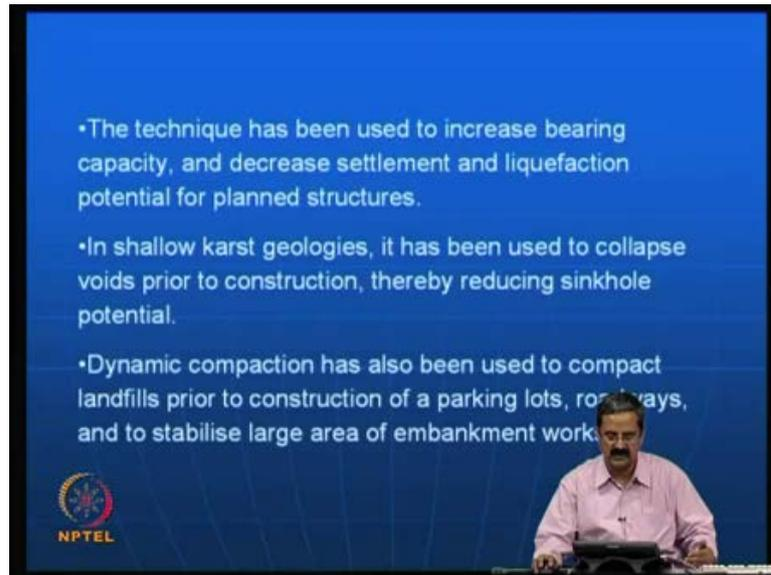
Normally, as treating granular soils and fills have always resulted in increased density friction angles and stiffness we will see this, how it can happen and as I just mentioned, this technique has been used to increase bearing capacity and decrease settlements in liquefaction potential for planned structures. In fact, this is one of the very important applications and in shallow karst geologies where this soil has a tendency to collapse it actually reduces the voids prior to construction.
