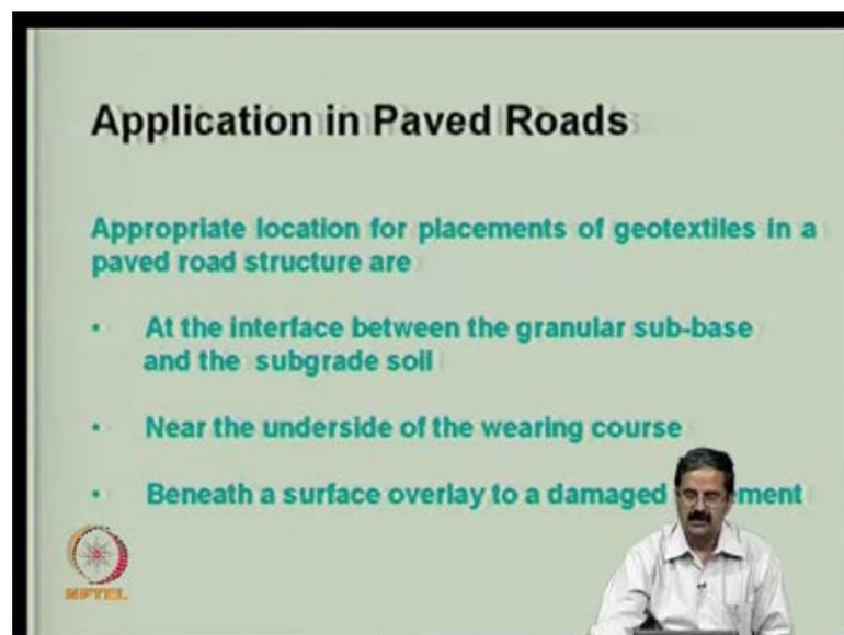
So, I also would like to highlight some more applications. So, the paved, unpaved road is that, where you are able to decrease the thickness of the pavement to some extent by using the concept of separation, and also one can use reinforcement. And if you think that the road drainage is a problem, you can do a filter design; and then, the most important thing is, once you do a paved road, what is next, you make you must make it paved, **right**; you have to have a wearing course.
