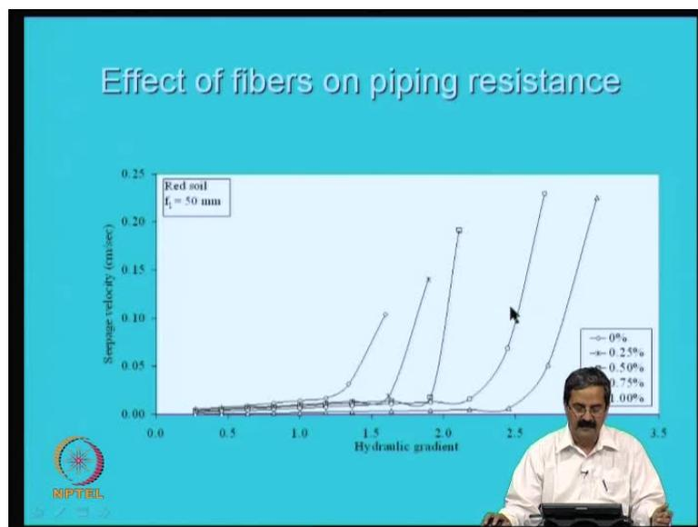
This is another important observation on piping resistance, the **many sands** many materials have quick sand condition like; you know, what is a critical hydraulic gradient? It is  $i_c$  equal to  $\frac{G}{1 + e}$  it comes close to about 1 and all that.
