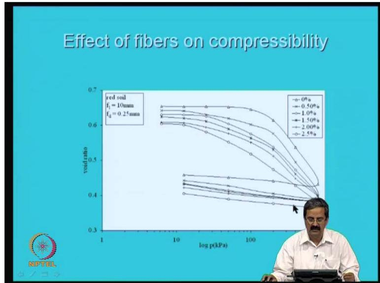
Then, you can see the effect of fibers and compressibility also, like why I am trying to cover just fibers is that they have been useful in all the applications. Like, you can see that originally the compressibility is quite high in the case of soil without fiber, but then, if we add fibers with increase in fiber content the compression index  $c_c$  and the recompression index  $c_r$  will come down, this is a very good advantage if you would like to reduce compressibility.
