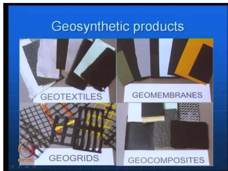
Then, these materials called geotextiles or geosynthetics, you have many types of products here, you have a geotextile here, you have a geomembrane here, you have a geogrid here, you have a geocomposite here.
