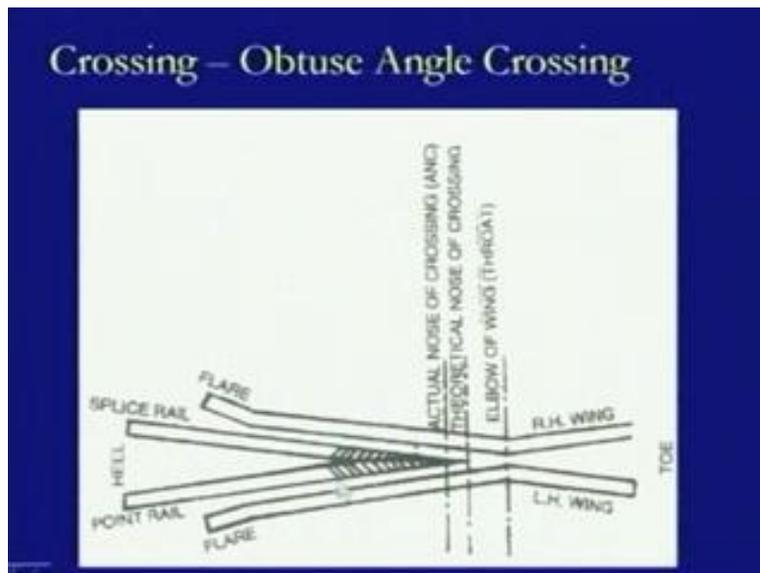
In this case, the obtuse angle crossing we just have a bigger angle which is formed and in that case that is what is this is actual nose and these all again are being shown in the same form with the throat.
