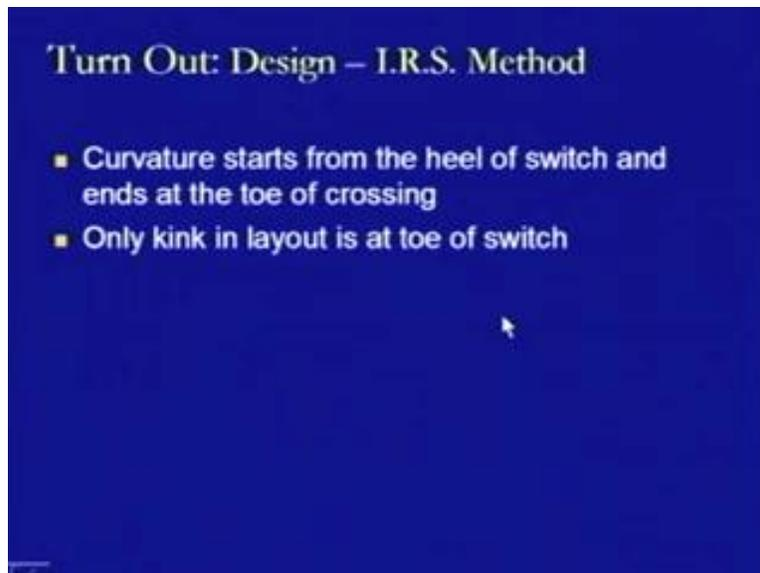
Now, we come to another method that is Indian railway specification method, I.R.S method mostly used on Indian railways. Here, in this method, the curvature is assumed to start from the heel of the switch and it ends at the toe of the crossing and only one kink is there that is at the toe of the switch. That is we are reducing the kinks slowly and slowly and making the operation smooth.
