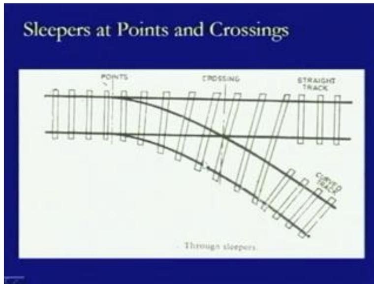
Then, this is another diagram, where the through sleepers have been shown and what we find is as we go forward like this up to the end of the crossing this size of the sleepers are required and that is what is a problem in this case. But then, this is a better way of providing the sleepers as compared to the previous one.
