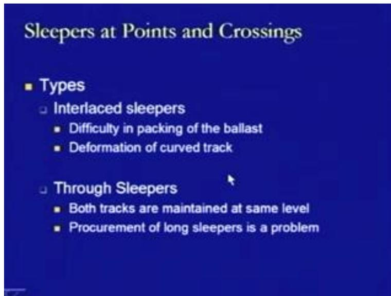
The interlaced sleepers - the interlaced sleepers are the sleepers which are provided in one track and then, they are being combined together from one track to another track in a form that they are coming alternatively for both the tracks. What happens in this case is
