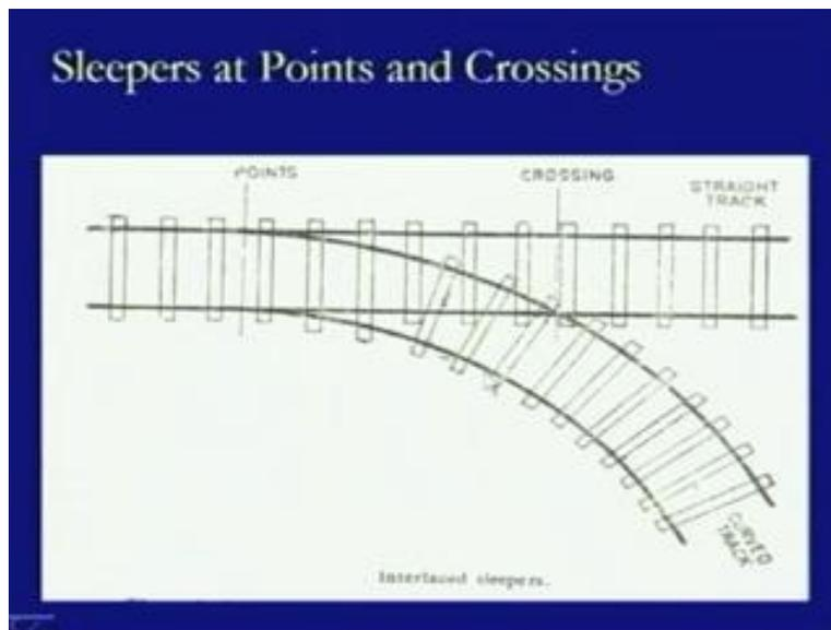
We will look at this diagram. This is the interlaced sleeper, where the sleepers are provided for this track and the sleepers are also provided for this track and then this sleeper is coming in between the other two sleepers. That is the problem of packing. You cannot pack the ballast in this area.
