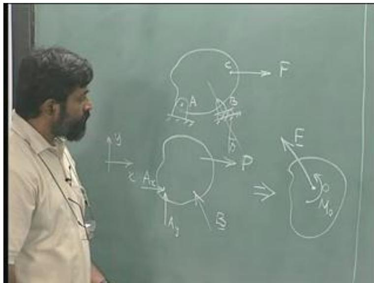
How do we write  $F$ ?  $F$  is nothing but we have these forces  $A_x$  acting along this direction plus  $A_y$  acting along this direction plus  $B$  which is acting along the direction  $\theta$  two
