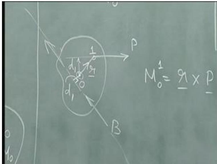
For example I am just going to erase this and draw fresh so that you can understand, how easy it is if I write it in terms of components. If this is the body, if I take this force p, I know this is a horizontal force. All I need to know is to find out the vertical coordinate difference between this point o and this point one. This y coordinate one with respect to o will immediately tell me that is the lever arm that I have to use to multiply with the magnitude of p.
