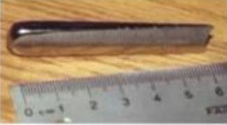
**A wedge of an amorphous Zr-Ti-Cu-Ni-Al alloy.**
