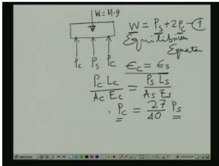
This is the bar or the block whose mass is  $M$  so the load that it transmits on those three bars equals the weight of it which is  $M$  into  $g$ . We have the three bars placed, central is the steel one and two copper rods, let us call the load that will be carried by steel rod as  $P_s$  and those of copper by  $P_c$ .
