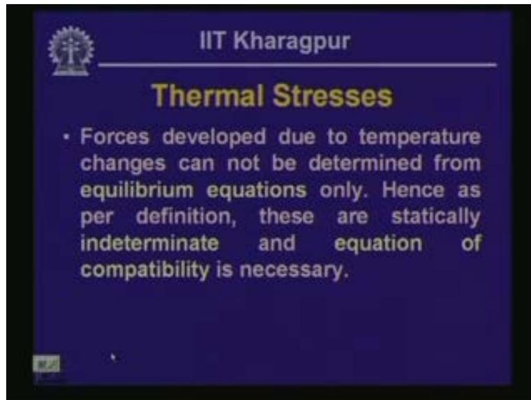
The forces developed due to the changing temperature, causes forces if they are restricted and these forces cannot be determined from equilibrium equations as we have seen earlier. Since we cannot determine the internal forces which are getting developed due to change in temperature, we call this kind of systems as indeterminate system according to the definition.
