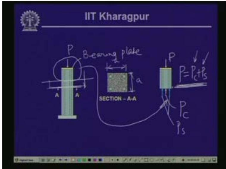
Similarly, here when the load is applied onto this member, the deformation of the concrete and steel, these two different materials which are placed in this particular diagram or in this particular member, the deformation of concrete and the deformation of steel should be same. If we say that the deformation of concrete is  $\delta_c$  this should be deformation in steel.
