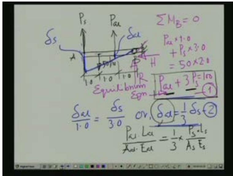
Once we note the steel rod and the aluminum rod they are subjected to the load  $P_s$  and  $P_{al}$  which we have evaluated. Hence we can compute that how much deformation this particular bar will undergo and how much deformation this bar will undergo. Since we are interested to evaluate the deformation of this particular point, if we know the deformation of this particular bar from this triangular configuration we can compute how much deformation this particular point will undergo.
