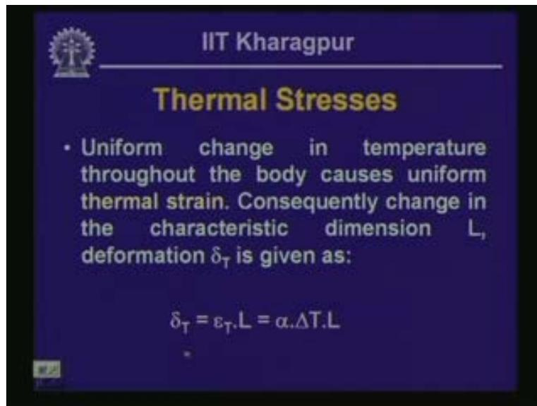
Uniform change in temperature throughout the body causes uniform thermal strain. This is important to know that there is strain which is developed in the body due to change in temperature; we call that as thermal strain.
