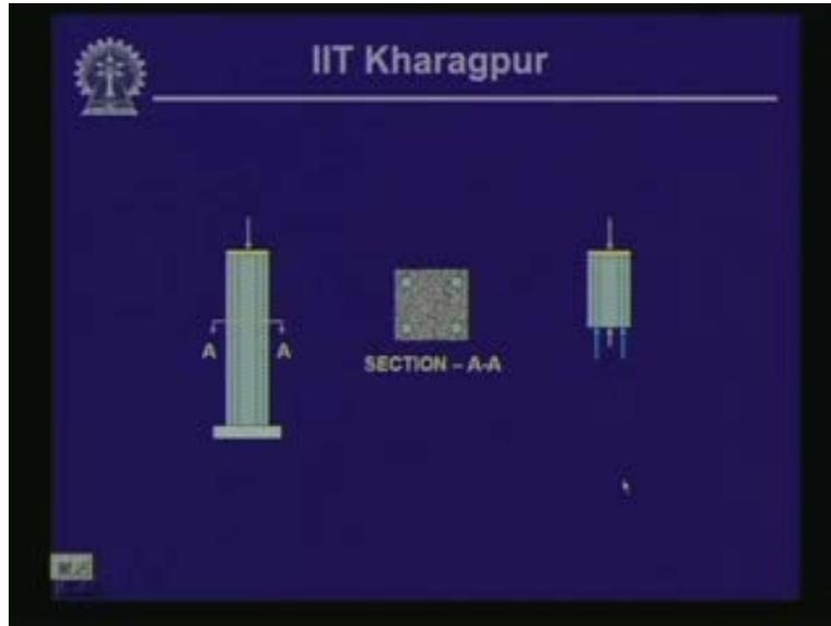
Let us look into this particular example which is quite common. You must have seen that the vertical members made out of concrete are provided with some steel bars if we cut a cross section here and look from the top then the section looks like this. Let us assume that the cross section of this vertical member is a square one with the sizes of the sides as  $A$ .
