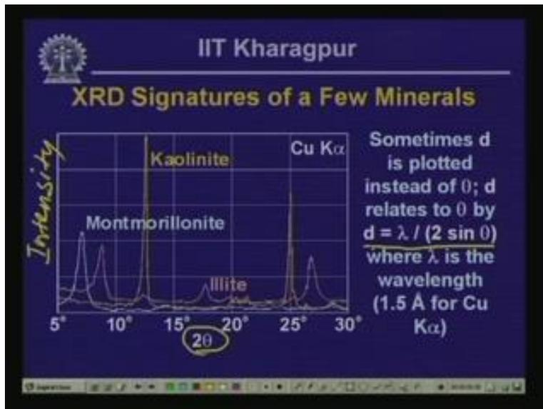
So, here we have got, we plot the angle and on the vertical scale, we have got the intensity of the X-ray signal and you can see at different angles depending on what mineral you are looking at, you are going to receive a very intense radiation. For instance, in case of Montmorillonite, you have got a radiation a signal, a peak signal appearing at 12 degree of angle.
