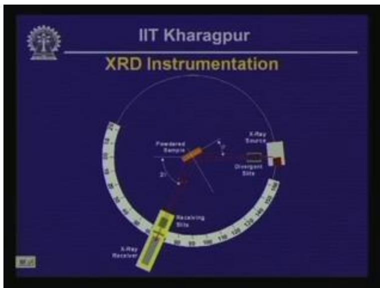
A schematic of an XRD instrument, X-ray diffraction instrument is shown on this cartoon here and you can see here what we have got is an X-ray source that actually made to impinge on a powdered sample, powdered crystal sample and then we have got a receiver that we can move actually along this graduated scale and we can note the intensity of the signal that is coming out of the powdered sample.
