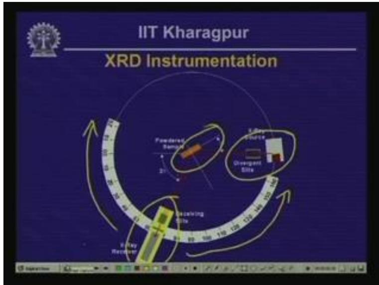
And, what we do actually? We plot the intensity of the received signal as a function of the angle and what we get in that process is this.
