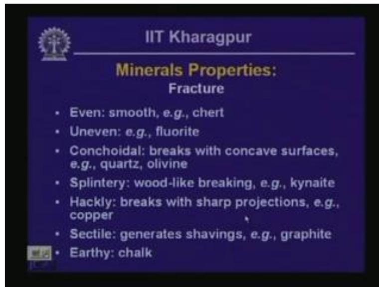
Now fracture, when you try to break a mineral, then the fracture could be smooth as we saw when we talked about cleavage, it is quite analogous to that type of property, here you have got a smooth fracture. And, when we talked about cleavage plains, we talked about eminent cleavage for instance, then fracture could be uneven. When you have got uneven fracture, then the surface in which the mineral aggregate breaks is going to be uneven as the name suggests.
