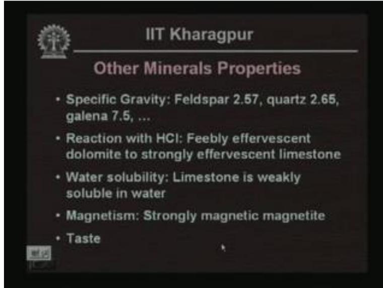
For example specific gravity of feldspar is 2.57; on the other hand, galena could have a specific gravity as high as 7.5 because of the presence of lead within the chemical, in the chemical composition.
