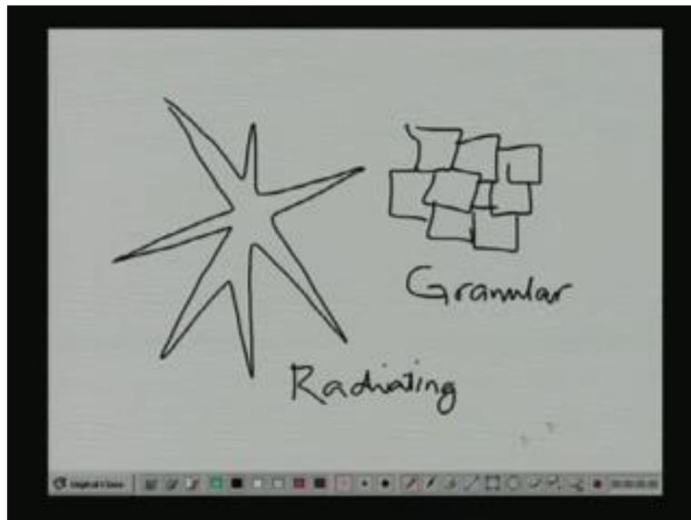
The matrix starts appearing like an assemblage of different grains. So, this one is a granular structure. So, that kind of takes care of different types of crystal forms. There are several other types of mineral properties that also allow minerals to be distinguished from each other one of which is specific gravity.
