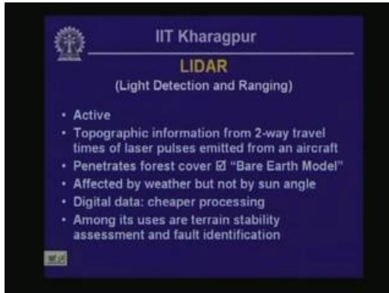
And, from the two way return time of the signal, one could develop the topography of a particular area as well as the nature; whether there is any vegetation cover or not from these two way return time of the LASER pulses.
