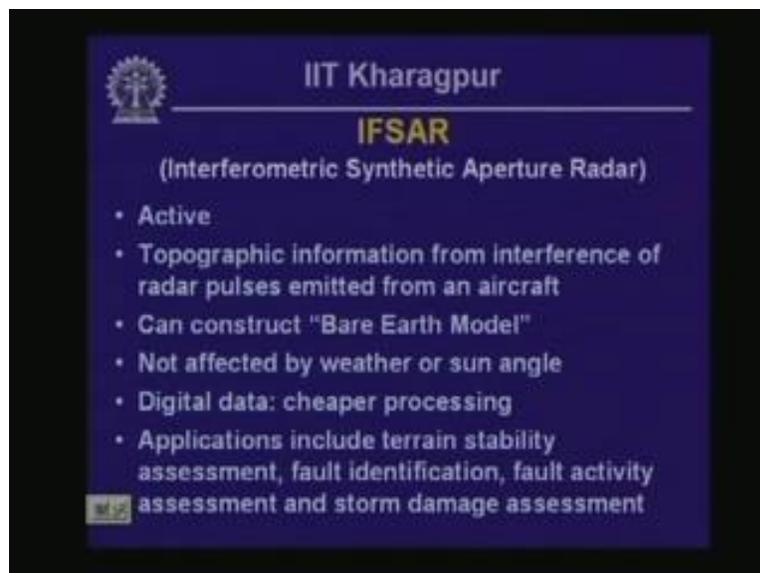
This is also another active remote sensing procedure and here, what is done is we use the interferometric principle to develop the topographic details of a particular area and again, both LIDAR and IFSAR, they can be used to construct a bare earth model that means if there is a vegetation cover, we can formulate a topographic information of the surface of the earth that is underneath the vegetation cover.
