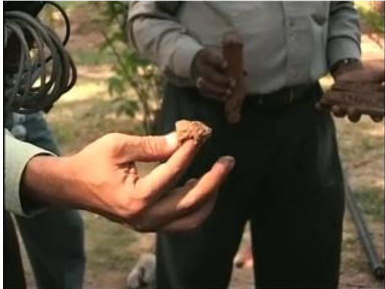
So, this sample is saved for grain size distribution and finding out the natural moisture content of the specimen. That is it.
