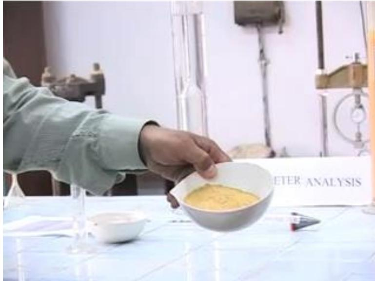
And what we are going to do with this particular sample is we are going to prepare a slurry of this particular soil sample, which has got, for which we want to find out the grain size distribution by taking 50 grams of the soil and making it mixing it up with water to make slurry of approximately one, exactly one liter. And we are going to place it, place the slurry making sure that soils are not readily settling in a sedimentation jar.
