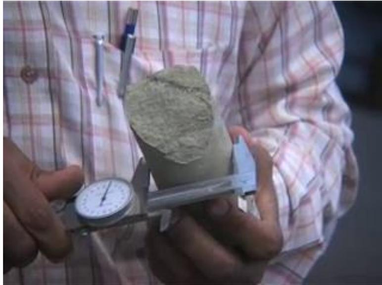
So, this sample, although it was obtained using the same reading, similar very similar reading, that similar reading equipment, the diameter is slightly larger than the one on my left hand and that is because of the durability of this sample. This, the sample that I am holding in my left hand is slightly more friable and slightly less durable than the one that I am holding on my right hand here. all right. Now, let us do the testing.
