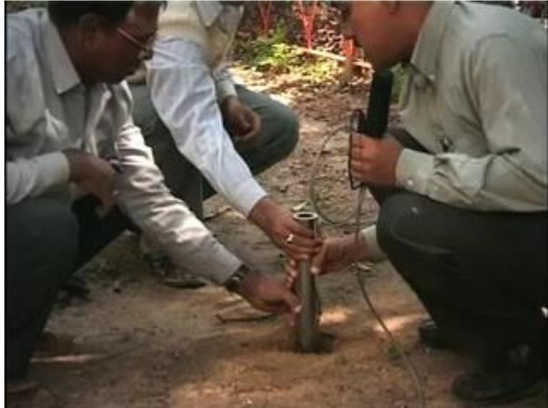
So, now, we have got the setup into the ground and what we have got here is a standard spt hammer mounted on the spt rod.
