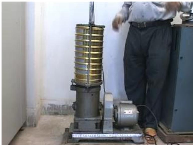
Now, you see that we have put the sieve set that you saw earlier, on which we took 500 grams of soil sample, on the mechanical shaker and we are going to subject it to mechanical shaking for about 10 minutes and after that we are going to find out what is the weight of soil retained on each individual sieve. And from that we are going to construct the grain sized distribution. So, just we will start the shaking now. You just watch it and then we are going to come back .
