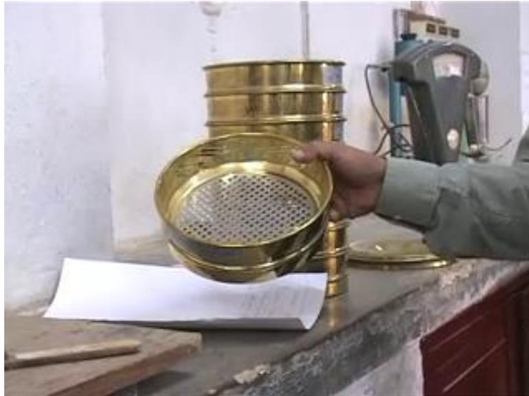
So, you see now after shaking of 10 minutes, we got the sieves back and as you recall that this was the coarsest sieve and in this one we do not have any coarse soil retained.
