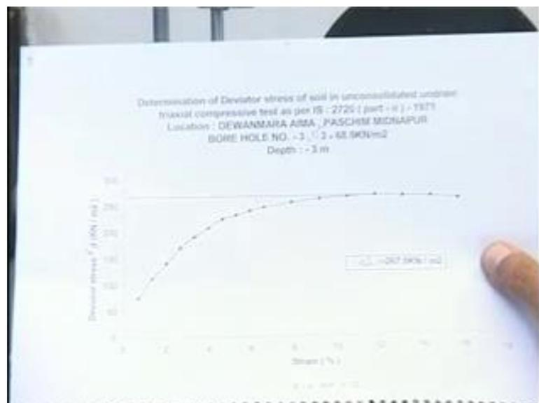
We prepare a plot of this type which is a plot of the axial stress minus the cell pressure that gives us the deviated stress, in this particular case, versus the axial strain. And as I was mentioning before we read the slope of this particular plot and that is, that gives us an estimate of that. From that, we can get an estimate of the undrained shear strength of the sample.
