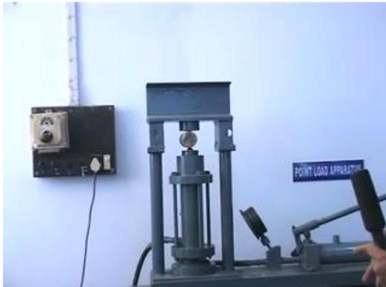
The sample is in between two points. You just observe the sample. It is going to crack once the point load reaches the failure value; the sample failed and the reading was roughly about 14; 14 kg per square kg per square centimeter at which the sample failed.
