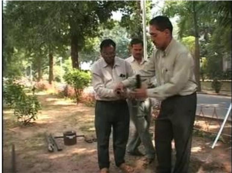
So, this is the cutting shoe which comes of like that and then the socket which connects the sampler to the spt rod. That also comes from the other side and then the portion in between splits into two different parts as you are going to see in the next little bit. You need a rod to do that and this is the two portions which split up like this one.
