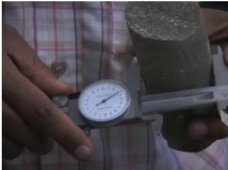
So, the sample diameter in this particular case is 53.36. I want to take a few more readings. So, here I am getting a value in this direction. In other orthogonal direction, I am getting a value, different value. Here it is 53.26. So, by taking such measurement in at least four orthogonal directions, whatever average diameter you get, you need to use that average diameter in your point load index calculation.
