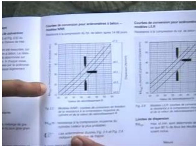
And then this value gets converted from a standard chart which is also given by the manufacturer. You have to read off the value of the ucs from looking at the appropriate curve.
