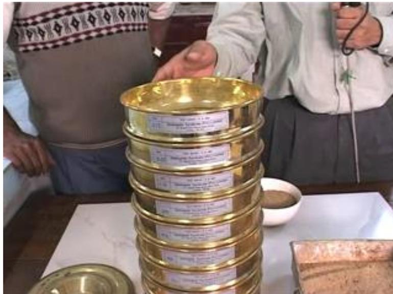
These are the higher standard sieves used for finding out the grain size distribution, as I was saying before, for coarse grained soils. What we have got here is a stack of different standard sieves which has got different opening sizes mentioned on the labels here. And you can see the opening of individual sieve from this pore set sieve that is being shown now and we can show now what is the appearance of the finest sieve used for finding out the grain sized using sieve analysis.
