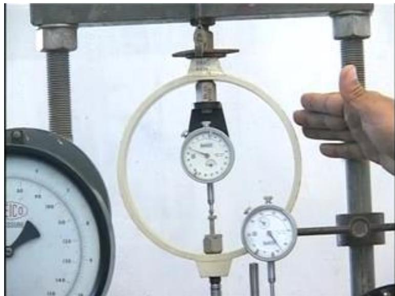
Now, we need to measure the axial stress on the triaxial sample for which we make use of a proving ring here and that is calibrated in such a manner that from the reading on this particular dial gauge, we can find out what is the stress, actual stress on the triaxial sample. Then we have got the displacement. We make use of this particular dial gauge for finding out what is the axial displacement of this particular triaxial set up.
