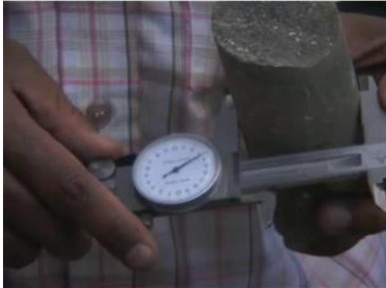
So, here again we are getting a readings of roughly 53.26 millimeter. all right. So, let us say, let us say the diameter of this sample is about 53.3 millimeter and we are going to use that 53.3 millimeter in our point load index calculation. So, this one, this sample here is 53.3.
