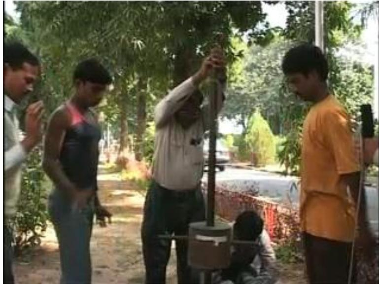
So, you see that the first 150 millimeter penetration is completed with only one blow; the soil is quit soft here. Then we are going to go with the next penetration of 150 millimeter.
