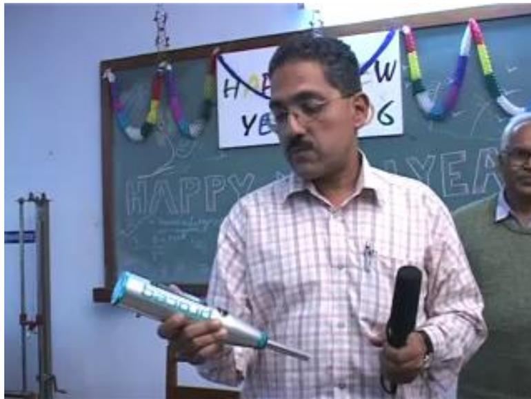
This is the instrument that we are going to use for nondestructive testing of a rock mass. It is very simple index really. So, what happens here is that we are going to push the instrument in and we have to make sure that this particular knob is stressed when the rebound occurs in order to measure the rebound value and the reading is going to appear on this particular scale here.
