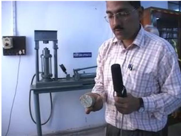
So, this is the face where the sample broke and we are going to record the point load, actually the pressure which is 14.7 kg per square centimeter at which the sample failed. So, I am recording it here.
