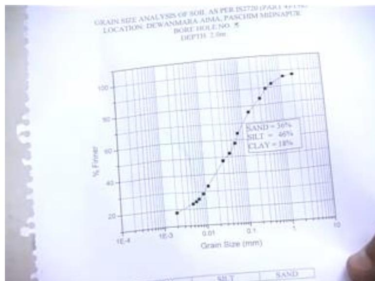
Finally, using the data, we are going to be able to generate a distribution, grain size distribution curve like this which plots the percent finer by weight on the vertical scale and the opening size of the sieve on the horizontal scale, as you see on this particular plot. So, using that we get a, we construct a grain size distribution and this allows us to classify coarse grain soils as I indicated earlier in one of the theoretical sessions in the course.
