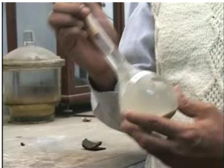
So, here you see that the soil is kept under a vacuum pump kept under vacuum here and that is being shaken by my colleague here, so that the water, so that the mixture does not have any intrusion of air because that might actually, as I was mentioning that might, introduce some error in the estimated specific gravity of solids..
