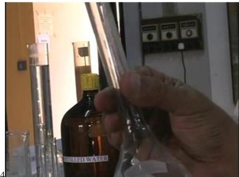
In fact, this particular flask is calibrated to be of 250 milliliter of volume at 27 degree Celsius and you can see that there is a mark on the stem of this particular flask and we are going to take distilled water exactly up to that mark. We are going to find out what is the weight of the flask plus distilled water and then we are going to take the distilled
