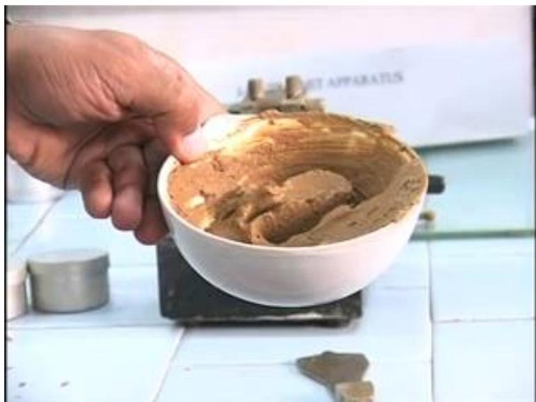
And what we are going to do? We are going to make a pat of this particular soil sample in this pan here.
