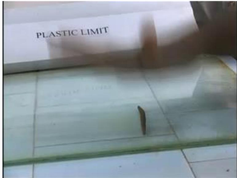
And this is the pat of the soil that we that we have here and we just try to roll a thread by the procedure like that, and you can see that as the thread becomes finer and finer, it will have a greater likelihood of cracking. So, here we have got a thread which is probably about twice as thick as the standard 3 millimeter diameter piece of wire here.
