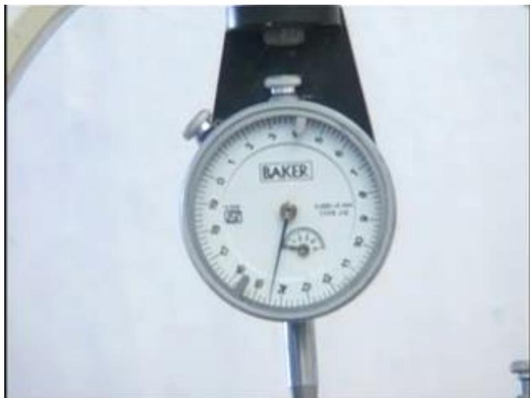
You can see that the loading range here is gradually decreasing. In other words, it is taking more and more movement to mobilize a certain amount of soil reaction. It is virtually stand still; it is not increasing any more. So, we are going to terminate the test
