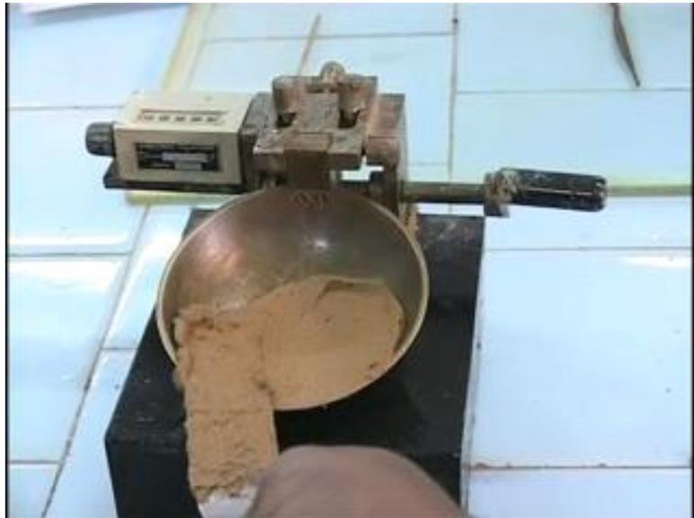
So, now, you see now we are preparing the pat in the pan making sure that there is no air entrapment within the volume of soil and the surface of this particular pat should be approximately horizontal. And then we use the grooving tool, as you see here, to cut a groove at the center of the pat, of the clay pat or pat of fine grained soil, and this is the groove that we construct, that we have constructed here using the standard grooving tool.
