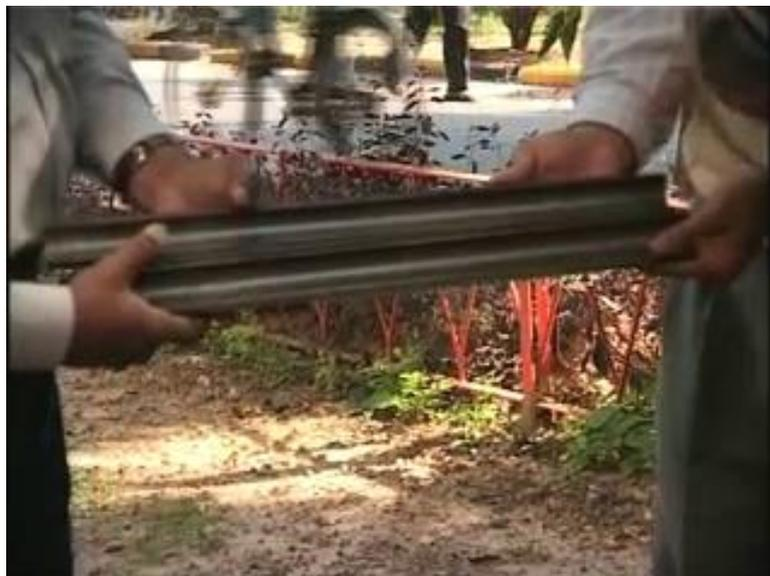
And then we assemble the stuff to and then then drive it into the ground to retrieve the soil sample. Now we can reassemble the stuff. So, this is how the sampler is assembled.
