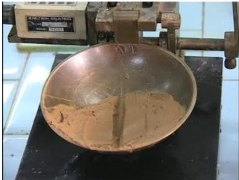
And you see here the pat is closed by an amount of approximately 12.5 millimeter and closure is approximately counted from there to about there and the number of blows in this case is much larger than 25. And what we are going to do? We have to keep on adding a little bit of water to the sample until we get the groove to close by 12.5 millimeter exactly on the 25th blow. And for doing that, what do we do?
