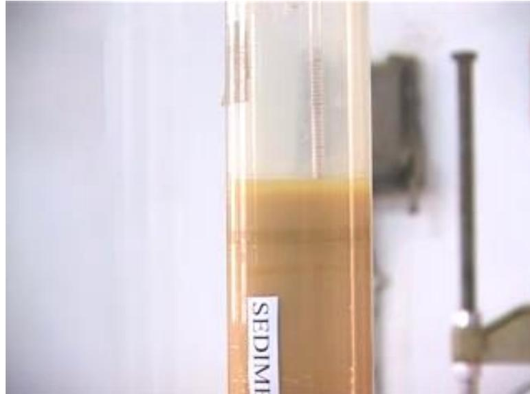
Now, you see that the hydrometer is being inserted very gently into the soil and what we are going to do? We want to make sure that the hydrometer does not bob up and down when the when it reached its equilibrium position. So, we have to be very careful with this thing and you can see the reading at the meniscus for this hydrometer position is about 1009 for the level for the water, for the level of the slurry that intersects the hydrometer stem.
