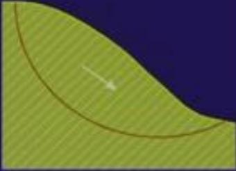
So, this is really a rotational landslide in which we are looking at a cross section of a slope underlain by relatively homogenous soil or rock. In this case in many cases, the
