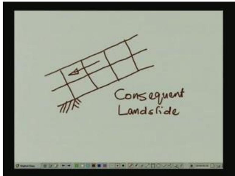
So, let us say you have got a slope where there are joint sets like this. This is a schematic picture of a cross section run through a particular slope, and the material underneath this jointed rock is massive and quite stable. And if this rock slides down slope in this manner, then this particular landslide is going to be called a consequent landslide, okay. So, then let us go and look at the other extreme.
