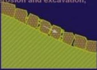
This is an illustration cross section really of the illustrating the process of block sliding. So, here what you see is pieces of rock, they are mobilized down slope near the slope face. This type of slide is called block slide.
