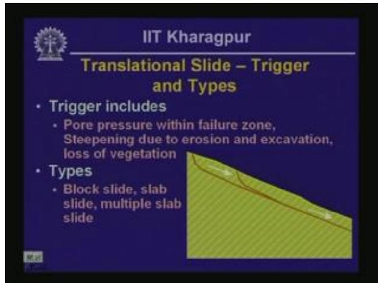
Slab slide on the other hand is like this. And there could be multiple slab slide where during sliding the slab that is sliding down slope that breaks apart in small pieces. So, these are the different types of translational slides.
