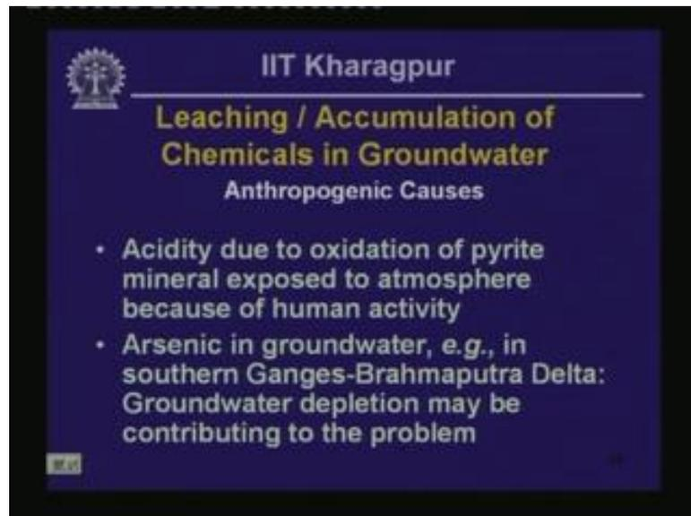
Or leaching or accumulation of chemicals could take place in groundwater because of anthropogenic causes because of human activities such as acidity due to oxidation of pyrite minerals. And that could happen in mine waste dumps, where the waste rock is comprised of pyrite minerals and oxidation of the pyrite mineral and leaching out and subsequent leaching releases acid in the groundwater.
