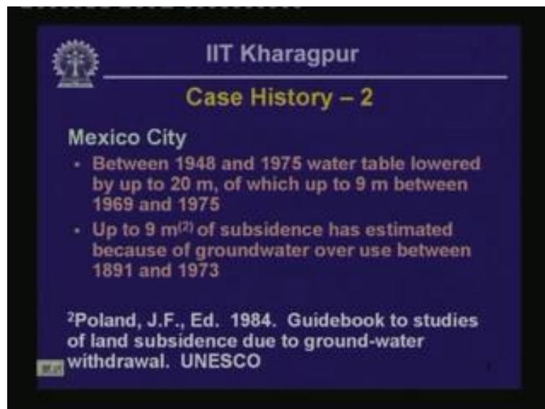
But the problem is more remarkable in another case history involving the capital city of Mexico. In Mexico city between 1948 and 1975, water table has been lowered by up to 20 meters. And out of these out of these 20 meters, 9 meter has taken place between 1969 and 1975. And unlike Calcutta, the soil condition in Mexico is comprised largely of fine grain material, but the fine grain soils are much softer remarkably softer in comparison with those encountered within the city of Calcutta.
