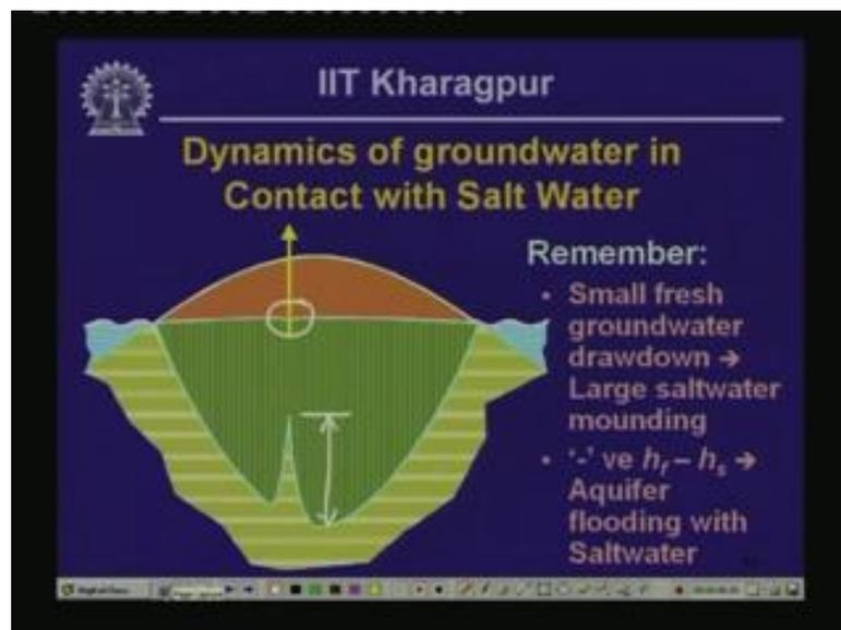
So, let us say we install water well at some location within the land mass within the land area and we start dewatering. And if we dewater leading to a slight lowering of water table, a remarkable salt water mound is going to form near the bottom of the fresh water wedge. And this you can see that this particular wedge is much larger actually, the height of this particular mounding is much larger in comparison with the tiny dewatering that we considered in this particular case.
