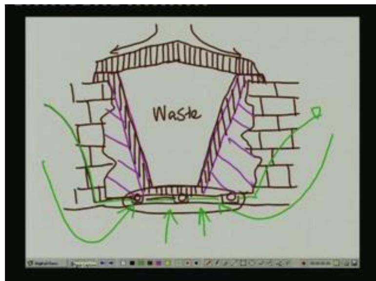
So, what we had there is an excavation within bedrock. This was, in fact, an original limestone quarry which got depleted got passed its economic use and then a landfill was constructed inside this particular quarry site, okay. Now if you recall what we had was a series of pipes at the bottom of the quarry itself. So, what these pipes do is to draw the groundwater table down to a configuration like this. So, let me use a different color pen.
