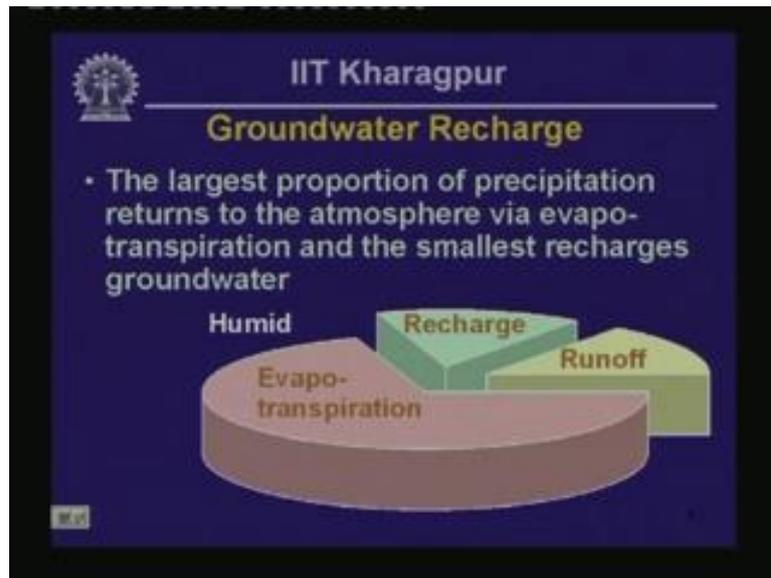
So, this pie chart here gives you the proportion that you could expect in a humid environment for recharge, and you can see here is that evapo-transpiration is approximately 70 percent of the total precipitation received in the area; approximately, 50 percent run, it is lost as runoff. Only fifteen percent is available to groundwater recharge.
