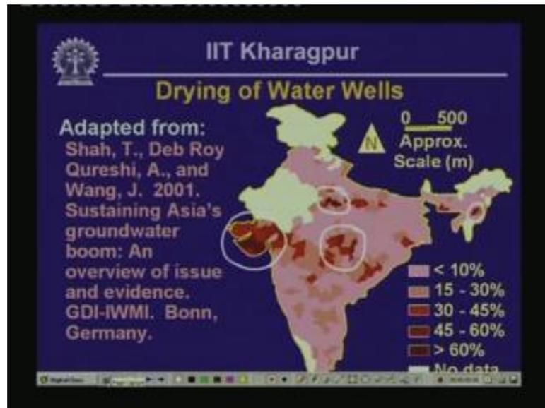
So, the first aspect that we are going to consider here is drying up of water wells. Now this particular slide shows you a map of our country, and it is basically color coded several areas within the country is color coded. And the deeper the color basically that shows the color coding is done in such a manner that deeper colors denote areas, where larger proportion of water wells have gone dry. And lighter colors are areas where only smaller proportion of wells has gone dry over recent years.
