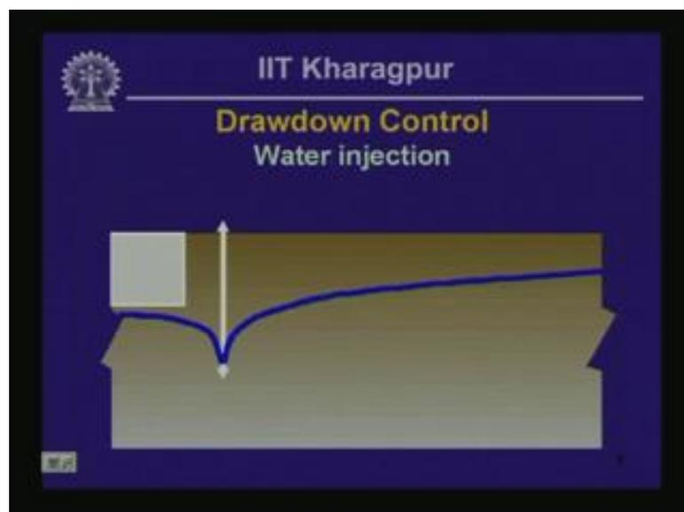
Now let us say in this particular problem we have to install a box like that. So, we are considering a cross section here a vertical cross section through the construction. So, this particular box is going to be partly submerged in the groundwater; the box could be of any purpose. It could be an underground garage or it could be in the form of an underground excavation that you are trying to open in order to construct some facilities underground.
