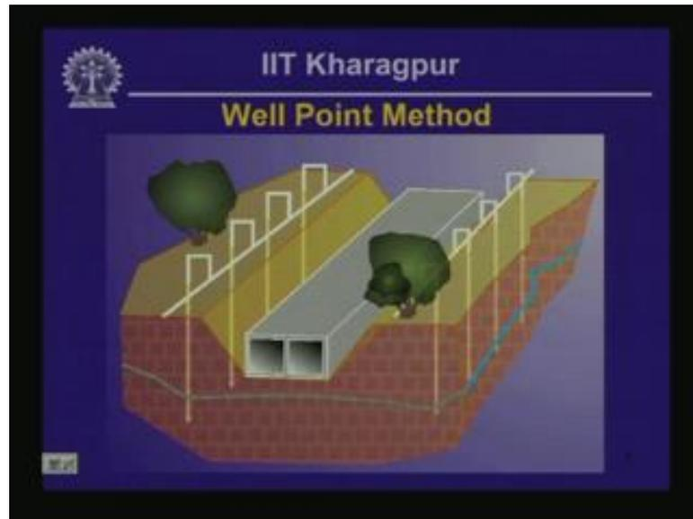
And then the box the tunnel can be installed or constructed inside the trench itself. And finally, what we are going to do is to back fill the trench.
