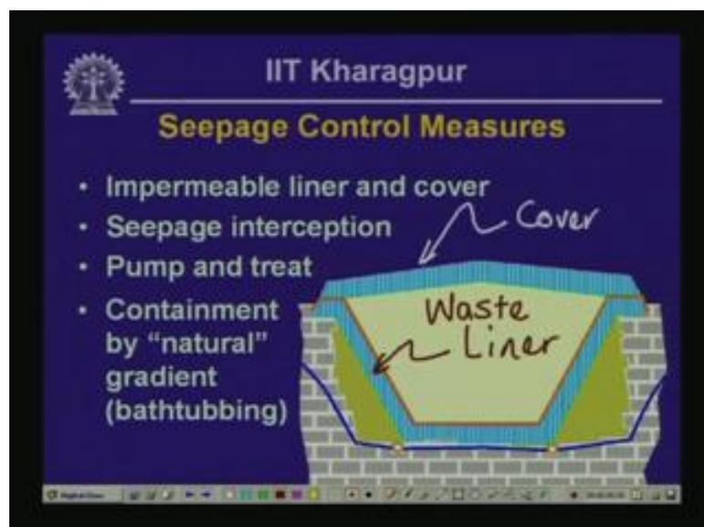
So, impermeable cover is this one; this is cover, and this one here is the impermeable liner. This is actually a cross section of a landfill that is constructed and was under operation near the Toronto Ontario Canada. Here what we have got this is the waste material shown with light off white shading, and the thick orange line here is a impermeable plastic material that is used in order to control a downward seepage through the waste material.
