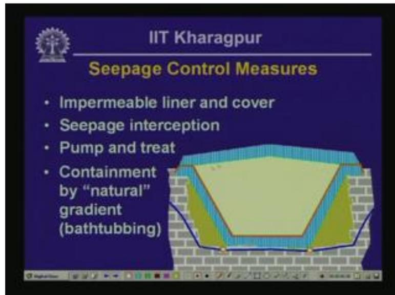
Seepage control measures include impermeable liner and cover. In this particular case impermeable liner and cover is indicated by hatched blue shaded area.
