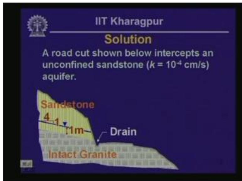
So, the question that I asked was - how much of flow will be intercepted on the drain that runs parallelly along the left edge of the highway shown on the cross section in the sketch there, and the problem was - the statement of the problem was - like this: the permeability of the sandstone aquifer was 10 to the power of minus 4 centimeter per second and what I have asked was, for you to find the design discharge for the interceptor drain. Now let us get on with the solution first.
