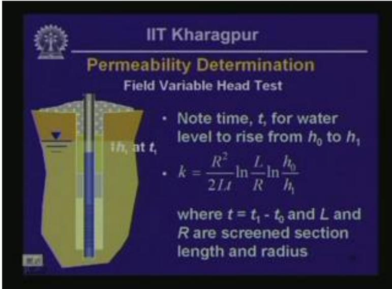
The slide features the IIT Kharagpur logo at the top left. The title is "Permeability Determination" in yellow, with "Field Variable Head Test" in white below it. On the left, a diagram shows a well casing with a screen at depth  $L$  and radius  $R$ . The water level in the casing is at depth  $h_0$  below the water table, and it rises to depth  $h_1$  at time  $t$ . On the right, the following text is displayed:
