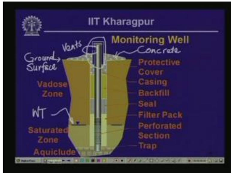
So, then you might ask - what is a monitoring well which is used in groundwater survey? A typical cross section of a monitoring well is shown on this particular sketch. So, it is essentially a casing, a tube - a casing tube - installed within a pre-bored hole, inserted within the pre-bored hole drilled or bored or excavated within the ground and the casing is shown at the center of the hole there, and you can see that there is a back fill around the casing.
