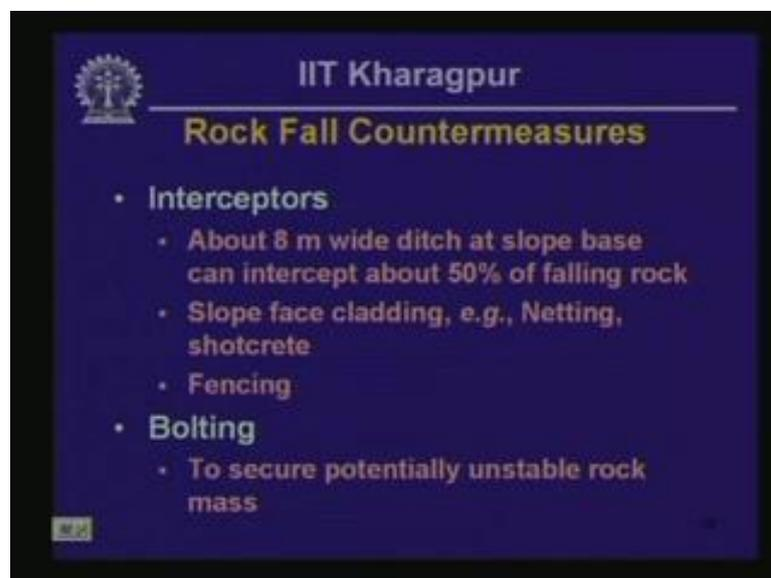
Rock fall countermeasures around road cuts, we can try to intercept the blocks of rock that might actually mobilize down slope. We could have a catchment ditch near the base of the rock. We could have cladding on the slope face in form of metal nets shotcrete facing, or we could have fencing parallel to the road cut parallel to the slope. These acts as barriers and intercept the falling rock or other debris or we could install bolting to secure potentially unstable rock mass on the slope face.
