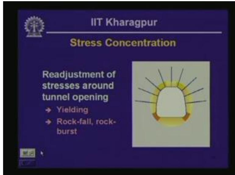
Okay, stress concentration is another issue that should be tackled while designing a tunnel. Readjustment of stresses around tunnel opening over and above its background value which developed over because of geologic processes may lead to yielding rock-fall and rock-burst. We discussed these topics previously. So, I am not going to get into the details of these things right now.
