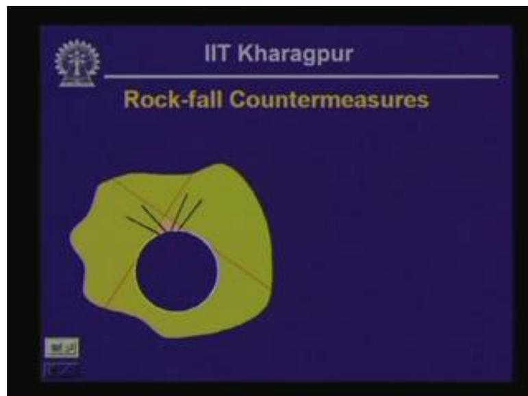
And we are going to construct a circular tunnel of that of that fashion. So obviously, in this particular case the wedge near the crown of the tunnel is going to be susceptible to falling over into the tunnel opening. And in this case we can stabilize actually this problem of falling wedge by installing rock bolts as we have just now discussed.
