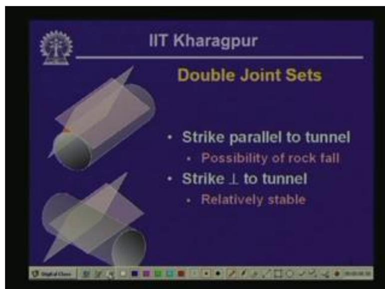
So, here again we are going to consider one tunnel let us say the tunnel alignment is like that, and the first joint set is oriented in that manner, and the second joint set is oriented in this manner. So, both these joint sets are striking parallel to the axis of the tunnel. So, in this case what is going to happen is that shaded area shown by orange shading near the crown of the tunnel is going to be susceptible to failure as soon as the tunnel opening is made.
