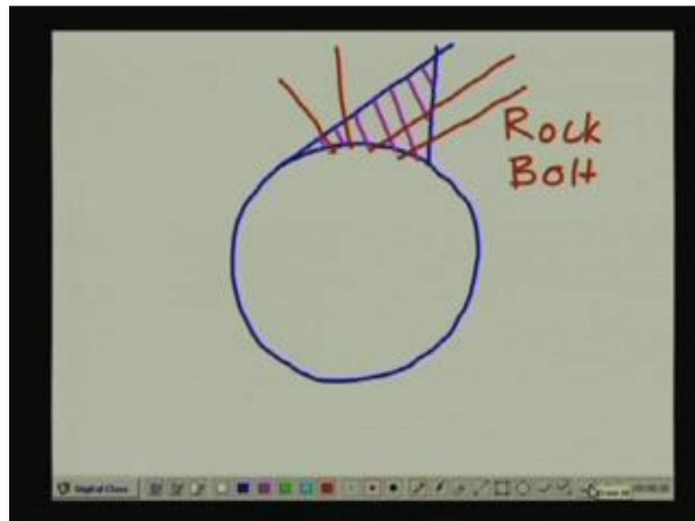
Let us illustrate this problem using a simpler configuration. Let us say let's revert back to the problem of the two joint sets striking parallel to the tunnel alignment, and let us assume that based on the principle of mechanics we have assessed that the wedge which is cross hatched with the purple color there is unstable. Then what could you do is to install rock bolts in this manner in order to stabilize this particular wedge and prevent it from falling into the tunnel opening.
