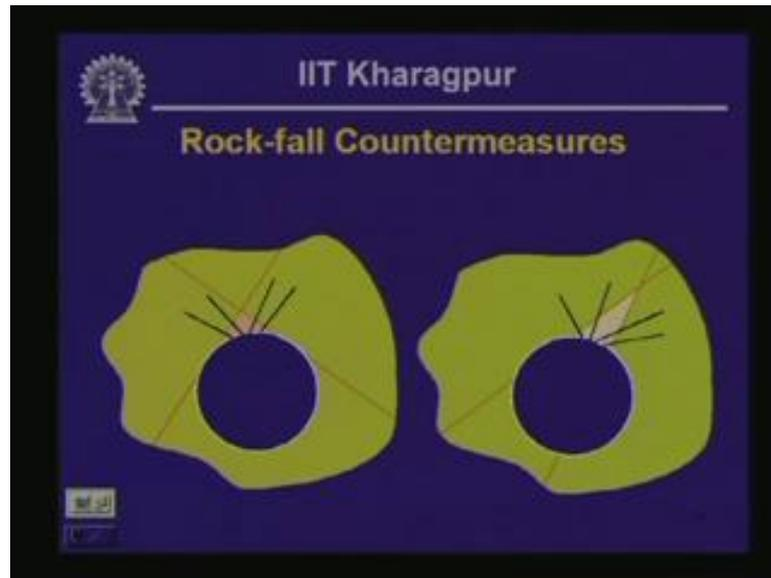
Now, another case which is the case involving involving a squid orientation of the wedge. Now here as I have indicated that the wedge is not always going to be unstable. You have to assess first whether the wedge is going to be stable or unstable. If you decide that the wedge is going to be unstable, then you can install rock bolts in order to stabilize this particular wedge from falling into the tunnel opening, okay.
