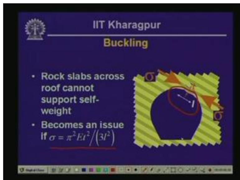
So, we are looking at the same tunnel, in fact, as in the previous case. And here again I have marked the direction of the major principle stress but by thick orange arrows. And it is quite obvious that as soon as the tunnel opening is made, then the slabs are going to buckle in that manner because of the removal of confinement near the top right portion of this particular tunnel. So, that is the area where the tunnel is going to be affected by buckling problem.
