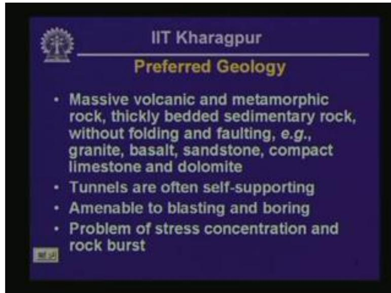
So, first of all what comes to mind is what is a preferred geological setting to construct a tunnel. And if you try to just look at the problem logically, then it would appear that if you have got a very strong mass of rock which is relatively free from joints or other structural features like shear zones or faults or rather fractures, it is relatively free from bedding or lamination. Then that is going to give us a very ideal situation to construct a tunnel.
