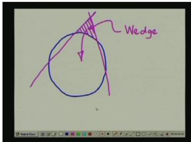
Let us say you have got a tunnel with a circular cross section as we considered in the previous slide, and you have got one joint set which is oriented in this manner. Then as soon as the tunnel opening is made then this particular wedge of rock, this particular
