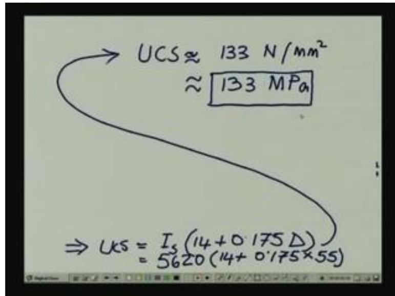
$$\begin{aligned} \text{UCS} &\approx 133 \text{ N/mm}^2 \\ &\approx \boxed{133 \text{ MPa}} \\ \Rightarrow \text{UCS} &= I_3 (14 + 0.175D) \\ &= 5620 (14 + 0.175 \times 55) \end{aligned}$$
