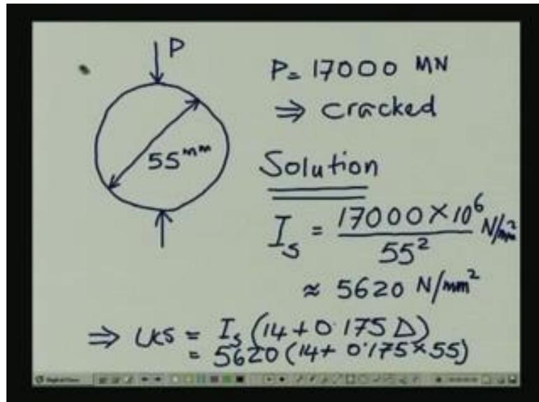
The image shows a handwritten diagram of a circular rock core specimen with a diameter of 55 mm. A point load P is applied to the top and bottom of the specimen. To the right of the diagram, the following calculations are written:
