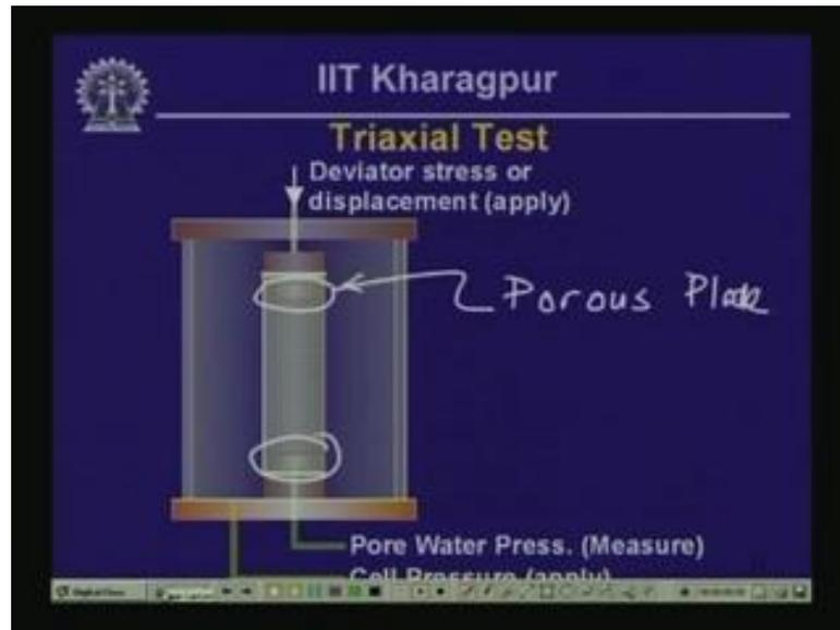
What you also should notice is that within the top portion, within the top pedestal, there is a porous plate and the use of that will be illustrated later and similarly, there is another porous plate at the bottom and that allows us to measure the pore water pressure within the element, and we are going to see, we are going to explain what is meant by that when we go further on soil and rock testing in one of the later presentations.
