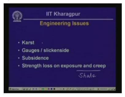
Then we look at the major engineering issues that affect the terrains underlained by sedimentary rock. Main problem here includes the terrains, limestone terrain, limestone terrain where portion of limestone can get dissolved in water leading to the development of karst topography and these types of areas are
