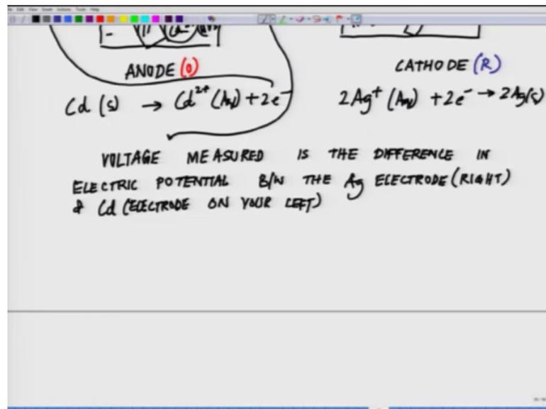
So, basically voltage measured is the difference in electric potential between the silver electrode that is on your right and the cadmium electrode that is on your left and cadmium electrode on your left. This is precisely how the configuration is and voltage tells us that how much work can be done when the electron is flowing from one side to another.
