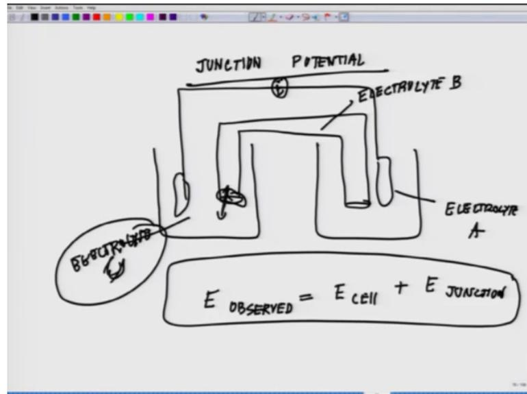
There is a concept which I wanted to introduce is called junction potential. What is junction potential? Junction potential is essentially, when dissimilar electrolyte solution are in contact. When dissimilar electrolyte solution are in contact a voltage difference called junction potential develop at their interface, this is a situation you will observe when you have a salt bridge, which has a different electrolyte, electrolyte B, and you have an electrolyte A, you have a electrolyte C.
