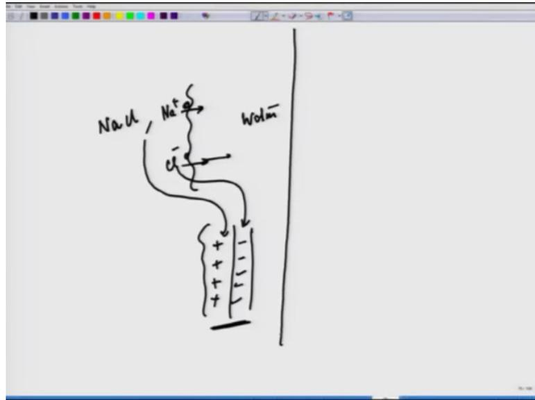
Say for example, you have this is the situation say for example, NaCl solution here, you have the water solution, and both Na ions and Cl ions are diffusing out both Na and the Cl ion begins to diffuse from NaCl solution into water.
