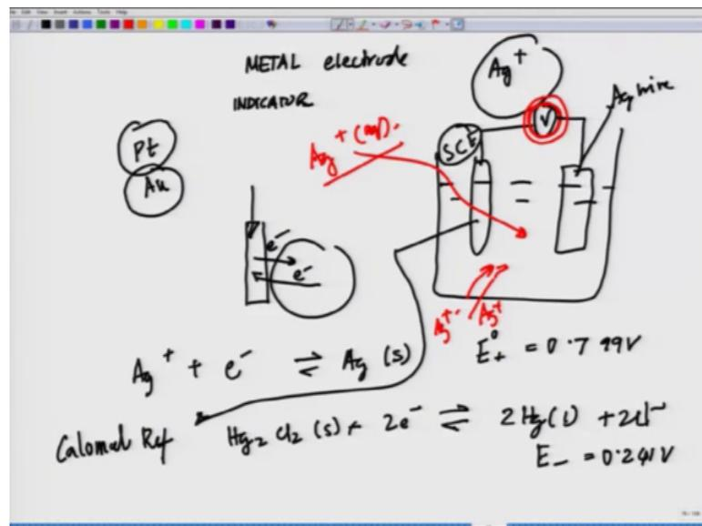
So, one of the metal electrode we will talk about today. Metal electrode is the one which is used for measuring Ag plus ion concentration. So, the most common metal indicator electrode. So, we have already talked about the reference electrode and the indicator electrodes. So, now we will be only concentrating on the indicator electrode of course, with respect to our 3 different kind of references either hydrogen or Ag AgCl, or calomel.
