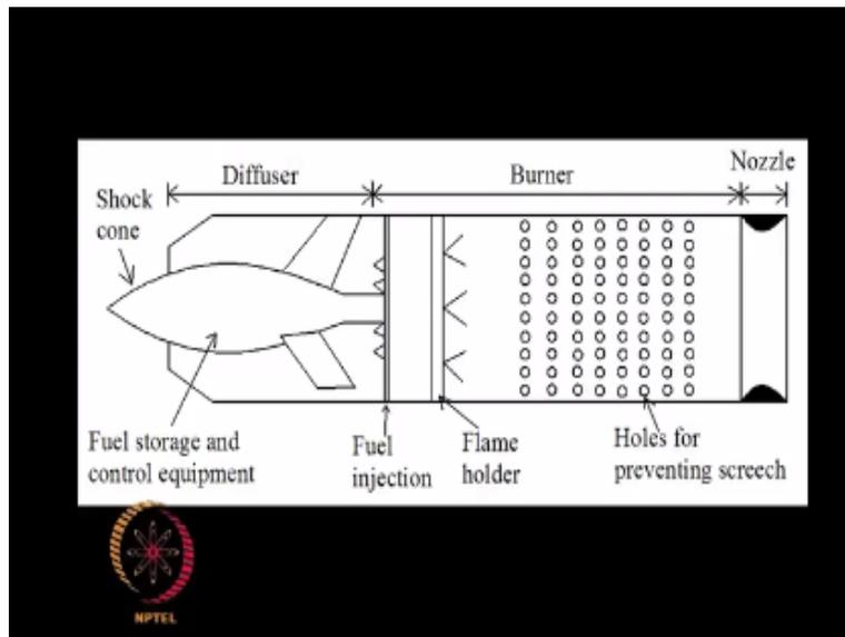
So if you see this figure here this is atypical schematic diagram of a ramjet engine, what you have here is a supersonic diffuser and then you have at this point the pressure of the incoming flow is already higher compared to the ambient pressure okay and then you have fuel injection here and the fuel flame holder here and the combustion takes place and then you have the flow expanding through the nozzle okay.
