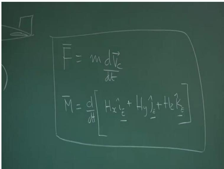
So what we did? We said we will also write equations of motion of an airplane. In fact to be more precise, we also know that we have to write perturbed equations of motion for airplane. Because these are perturbed equations of motion because these are measured from equilibrium when the perturbation was introduced. We wanted to develop such equation of motion which is a perturbed equation of motion for the airplane. But what was our approach? We said initially, we
