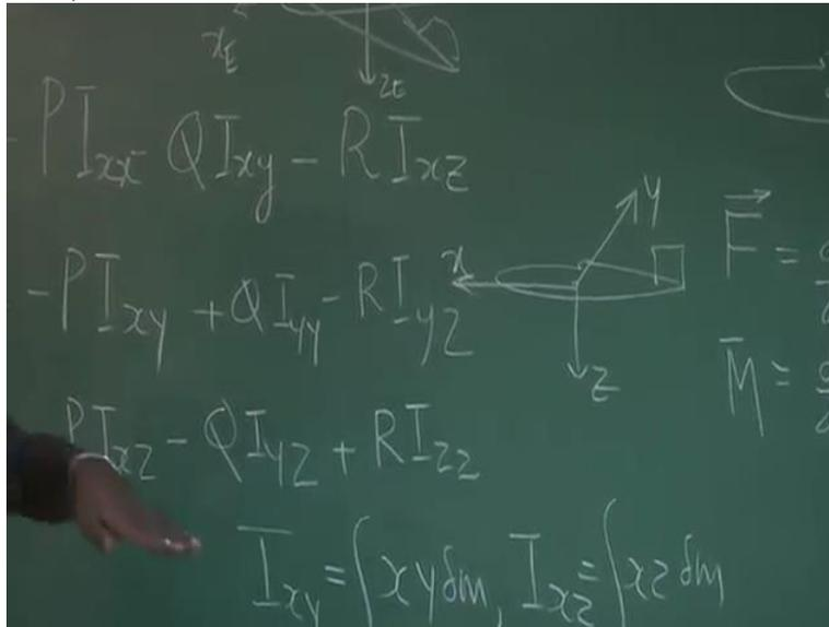
If I choose a body frame, if I am allowed to operate, knowing very well body frame is not an inertial frame, let us say X, Y, Z, body frame means, it is fixed with the body. And as the body rotates, this frame also rotates. So one thing is sure that moment of inertia now will not change about this axis because the axis is also moving. Then also, the aerodynamic forces will be proportional to the relative as speed. So along X, Y, Z, you can easily compute.
